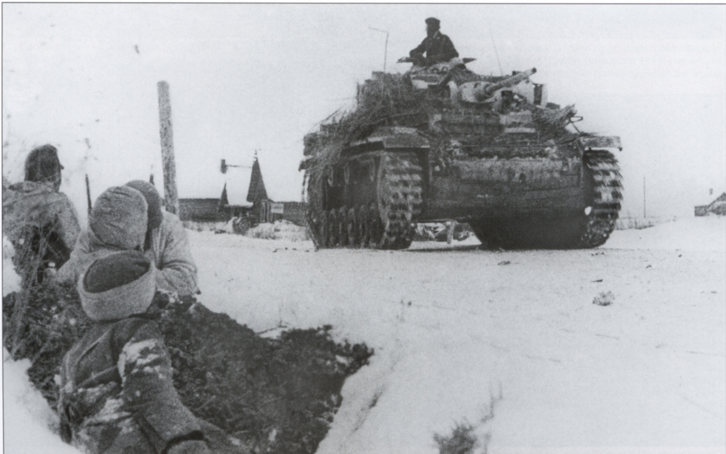
A heavily camouflaged Pz.Beob.Wg.III of a Panzer-Division's artillery regiment. The photograph was taken in January or February 1944, in central Russia. This particular model is armed with a dummy gun.
