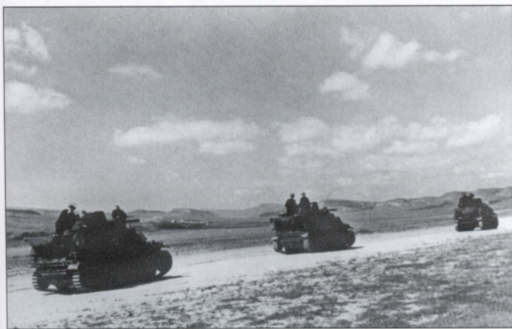
Two photographs showing the latest arrivals of Sd.Kfz.132 introduced into the Panzer-Divisions in 1942. These light anti-tank self-propelled guns were built on the LaS 138 chassis. They were armed with the captured Soviet 7.62cm anti-tank gun. In these photographs we see a number of these vehicles moving along a road somewhere in southern Russia. Throughout its service in the Panzer-Divisions in Russia the Sd.Kfz.132 was an effective mobile anti-tank weapon that was always on hand to provide infantry anti-tank support.
