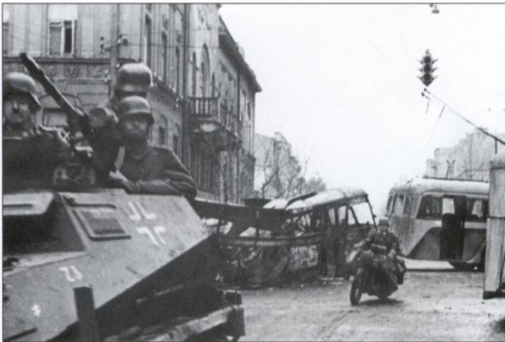
Sd.Kfz. 251/10 Ausf. A armed with 3.7cm anti-tank gun PaK36 leads an infantry troop during intensive fighting in the Kalinin area in late November. Note that the crew using sandbags around the gun shield for additional protection.
