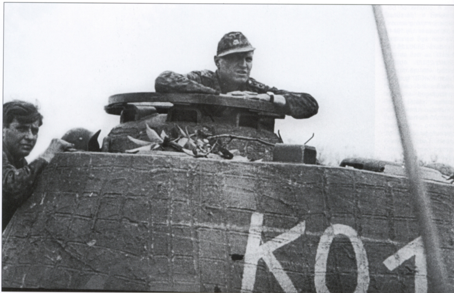
Two photographs showing Panthers belonging to the 5.SS-Panzer-Division 'Wiking' during operations near Warsaw in the autumn of 1944. The photos show the commander's tank with the tactical code 'K01' painted in white and applied over a coating of Zimmerit anti-mine paste.
