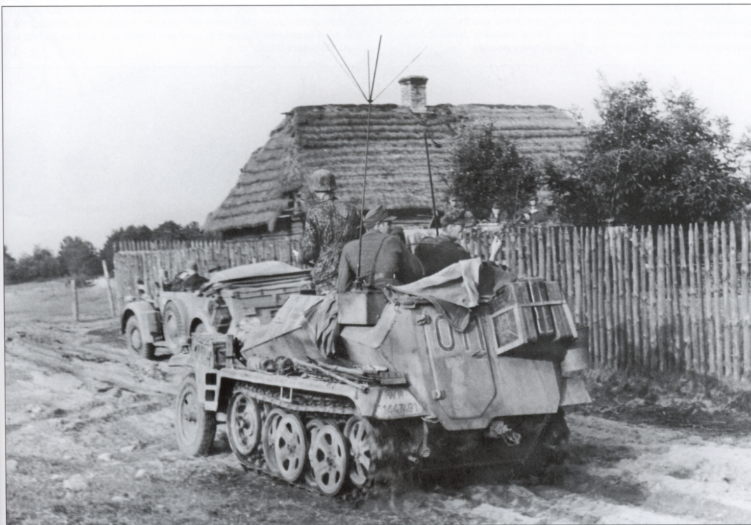
An Sd.Kfz 250/5 communication vehicle heavily laded with combat equipment during the autumn of 1943. The vehicle is painted in overall dark sand with a random application of green and brown camouflage wavy lines. It carries the staff markings, '011', probably painted in red with a white outline. On the license plate we can see WH144491. However, although this vehicle belongs to the Wehrmacht a Waffen-SS soldier can be seen on board.
