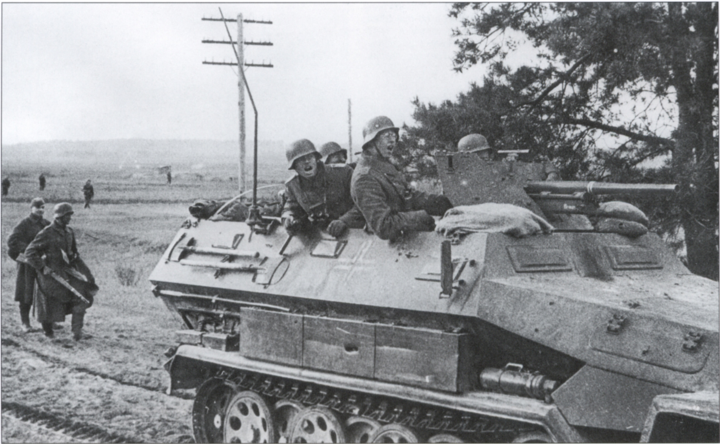
Sd.Kfz. 251/10 Ausf. A armed with 3.7cm anti-tank gun PaK36 leads an infantry troop during intensive fighting in the Kalinin area in late November. Note that the crew using sandbags around the gun shield for additional protection.
